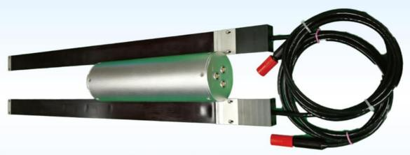
Shark-S150D side scan sonar (separated type) is versatile multi-purpose sonar which can be applied to shallow and deep water. It contains dual simultaneous frequency operation of 150/450 kHz and advanced CHIRP signal processing technology ,which provide extraordinary long range, high-resolution images.
